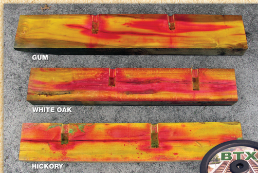
The penetration of borates into the wood is indicated by the red coloring of added curcumin.
